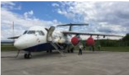
Figure 1. The Bae-146 of the Facility for Airborne Atmospheric Measurements (jointly operated by Natural Environment Research Council and Met Office) in the UK. This aircraft is comprehensively-equipped for measurements of atmospheric aerosols, cloud and precipitation particles, trace gases and radiometry from visible to sub-millimetre wavelengths
