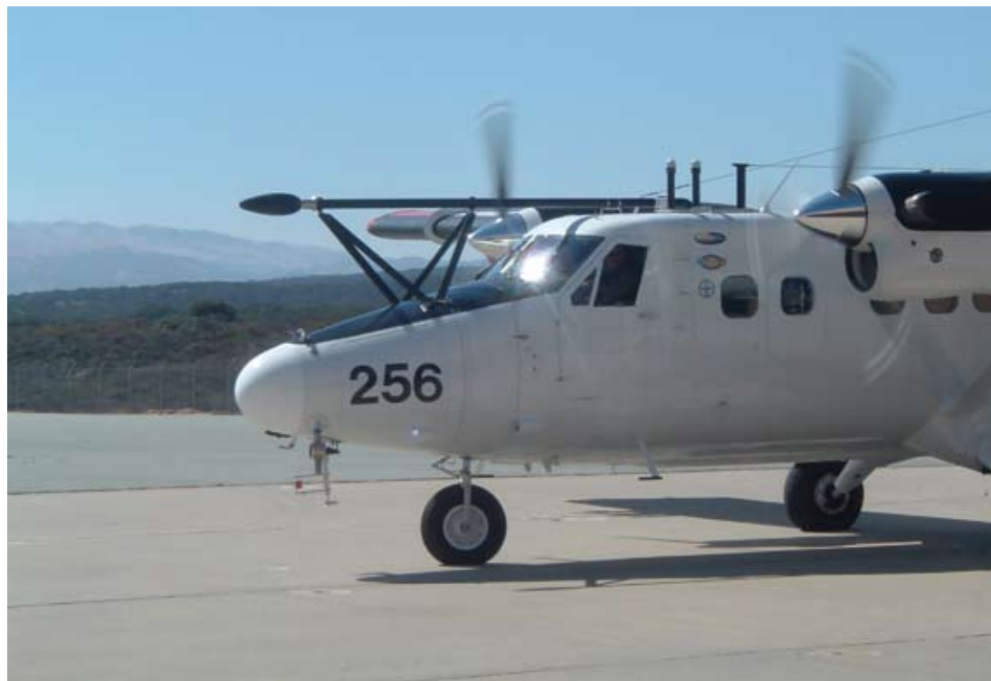
A research airplane carrying a UFT thermometer (red, below the tip of the fuselage) during the POST (Physics of Stratocumulus Top) experiment, California, summer of 2008
