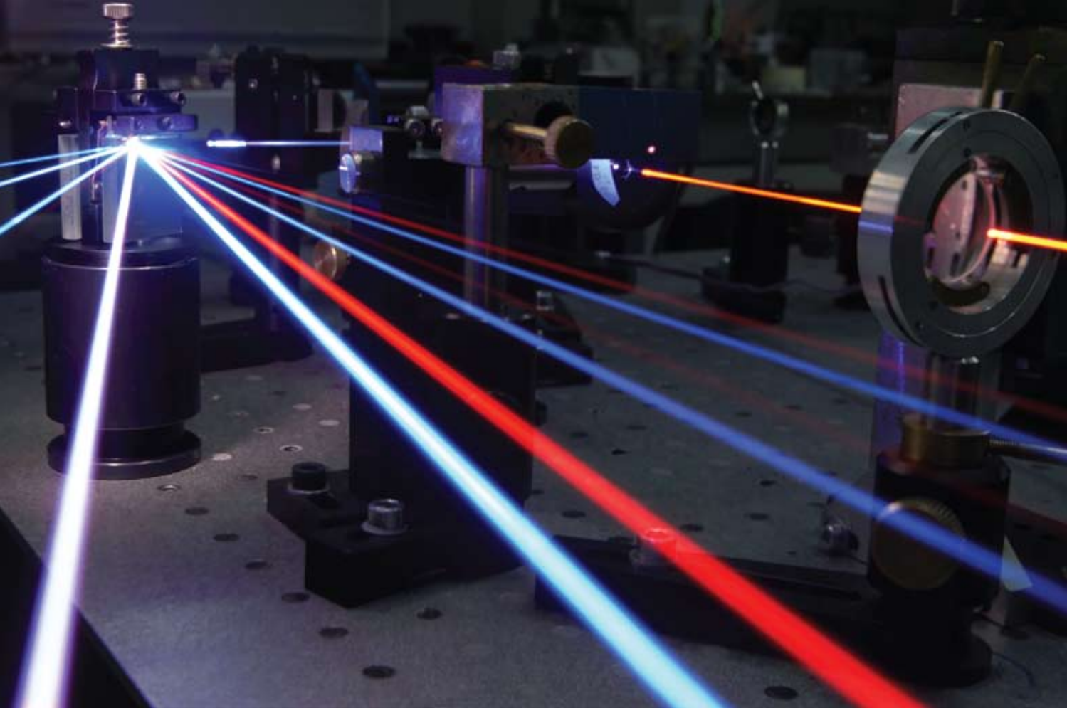
Generation of the second harmonic in a nonlinear crystal from a laser beam emitted by an amplifier of ultrashort laser pulses
