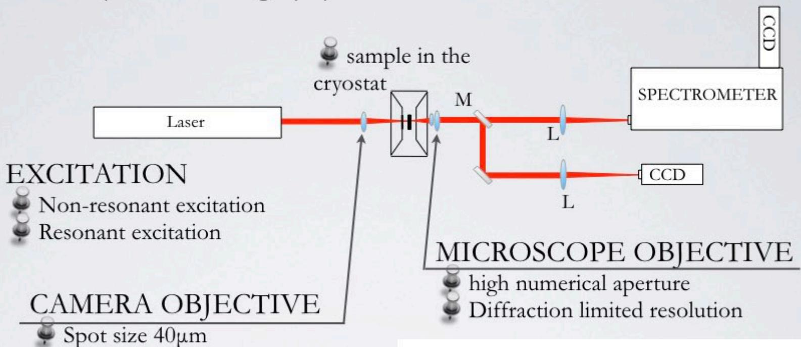
Imaging PL of the mesa on the slits of the monochromator.
