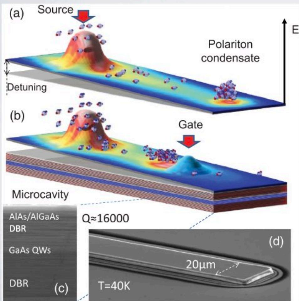
FIG. 1. (Color online) Schematic of the polariton condensate transistor based on a microcavity ridge (a) without and (b) with the gate. Scanning electron microscopy images (c) the cross section of bulk sample and (d) a  $20\text{-}\mu\text{m}$  ridge.
