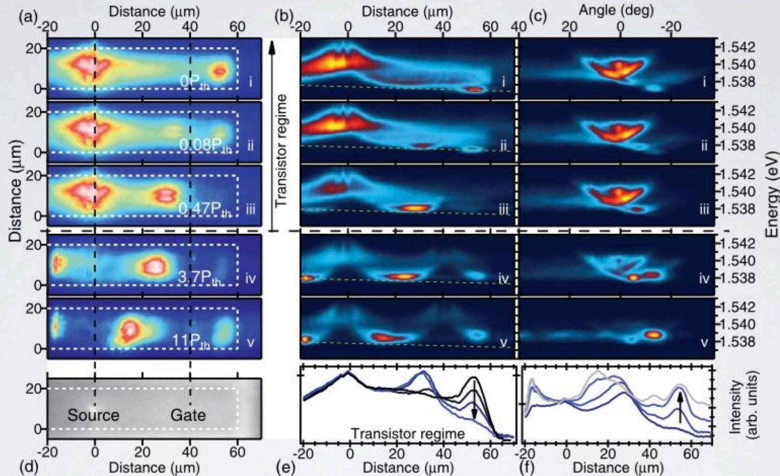
FIG. 3. (Color online) (a) Real-space, (b) energy-real space, and (c) energy-angle space images for different gate powers (i–v) for a constant source power ( $10P_{\text{th}}$ ). (d) White light image of the ridge showing the positions of the source and the gate. The line profile (log scale) along the center of the ridge for a gate power (e) below and (f) above threshold for increasing gate power (as indicated by arrow).
