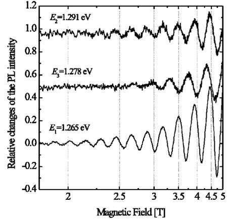
FIG. 2. Relative changes of the PL intensity  $[I(B)/I(1\text{ T})]$  from the modulation doped GaAs/InGaAs/AlGaAs QW with a high density of the 2DEG measured at  $T=4.2$  K at the PL cutoffs at the energies  $E_1$  and  $E_2$  as well as at an intermediate energy  $E_3$ . Linear background has been subtracted and offset has been added for more clarity.
