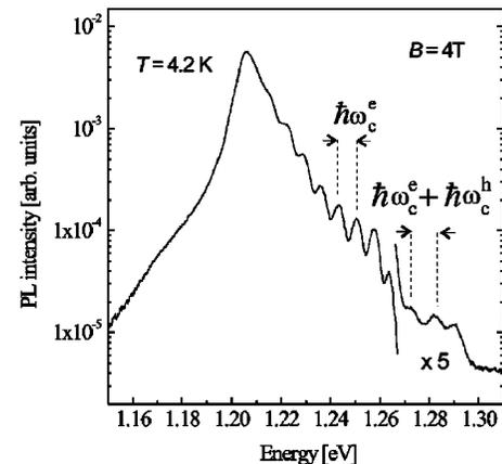
FIG. 3. Photoluminescence spectrum of the modulation doped GaAs/InGaAs/AlGaAs QW with a high density of the 2DEG measured at  $T=4.2$  K in magnetic field  $B=4$  T. Landau-level quantization with electron cyclotron energy  $\hbar \omega_c^e$  (a sum of electron and hole quantization energies  $\hbar \omega_c^e + \hbar \omega_c^h$ ) can be seen in energy range  $E < E_1$  ( $E_1 < E < E_2$ ).
