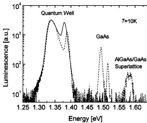
FIG. 2. Electroluminescence at  $j = 16 \text{ mA/cm}^2$  (solid line) and photoluminescence (dashed line) from the modulation Si  $\delta$ -doped pseudomorphic GaAs/InGaAs/AlGaAs heterostructure at  $T = 10 \text{ K}$ .
