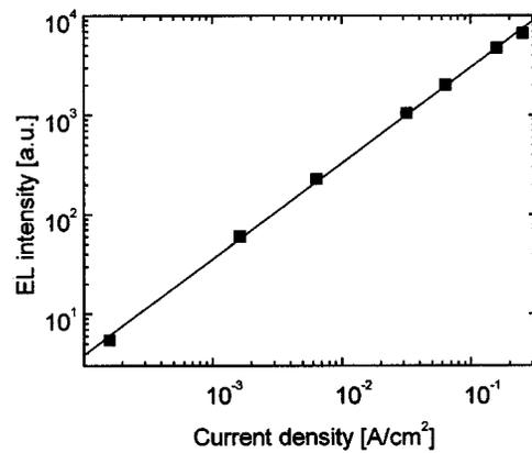
FIG. 3. Linear dependence of the integrated electroluminescence intensity as a function of current density at  $T = 4.2 \text{ K}$ .
