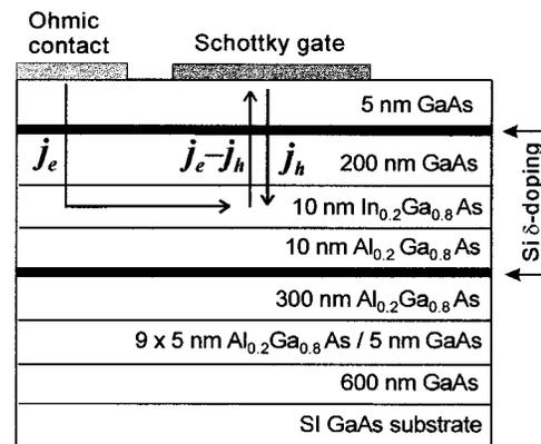
FIG. 1. A sample structure with schematically shown majority-carrier ( $j_e$ ) and minority-carrier currents ( $j_h$ ).
