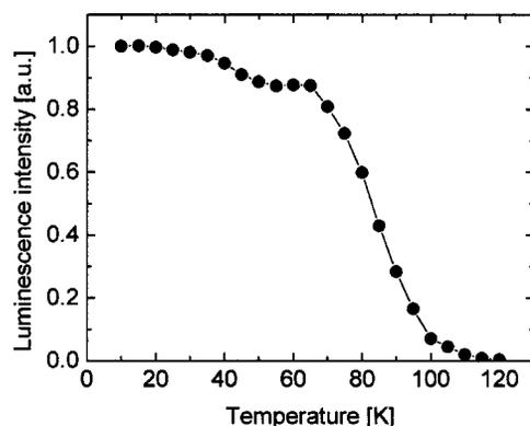
FIG. 4. Temperature dependence of the total integrated electroluminescence from the Schottky barrier diode on the modulation Si  $\delta$ -doped pseudomorphic GaAs/InGaAs/AlGaAs heterostructure at low temperature. Current density was equal to  $j = 16 \text{ mA/cm}^2$ .
