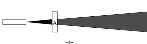
The function of filter  $A$  cannot be explained as a “sieve” that only lets those photons pass that happen to be already horizontally polarized. If that were the case, few of the randomly polarized incoming photons would be horizontally polarized, so we would expect a much larger attenuation of the light as it passes through the filter.
