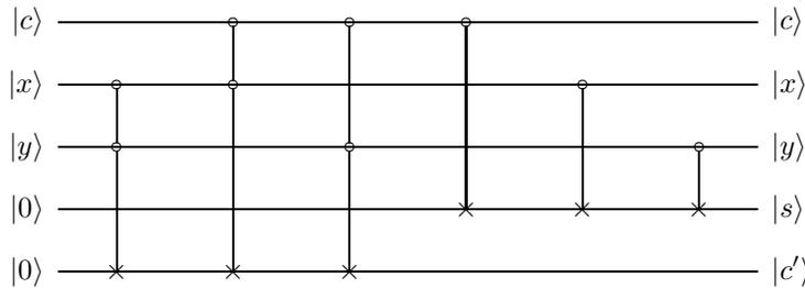
where  $x$  and  $y$  are the data bits,  $s$  is their sum (modulo 2),  $c$  is the incoming carry bit, and  $c'$  is the new carry bit. Vedral, Barenco and Ekert [Vedral et al. 1996] define more complex circuits that include in-place addition and modular addition.
