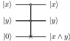
Now take as input a superposition of all possible bit combinations of  $x$  and  $y$  together with the necessary 0:
