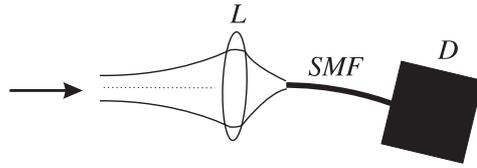
**Figure 1.** Detection of a quantum state of a single light-mode by means of a lens  $L$ , single-mode fibre SMF and a photon-counting detector  $D$ .
