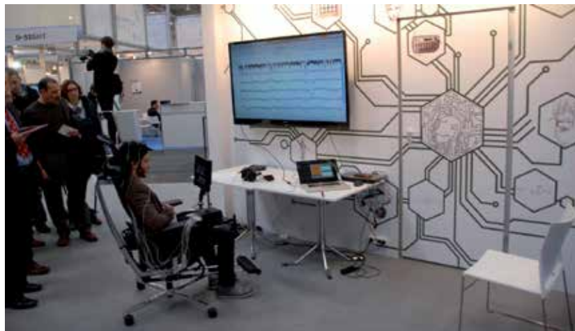
Figure 4. BCI Appliance presented at the CeBIT 2012 computer fair: tablet-sized box, connected wirelessly to the EEG amplifier, is attached to the armchair. Display on the wall plots the brain waves, analyzed in real time by the Appliance to detect the user's intentions – this element is only for demonstration
