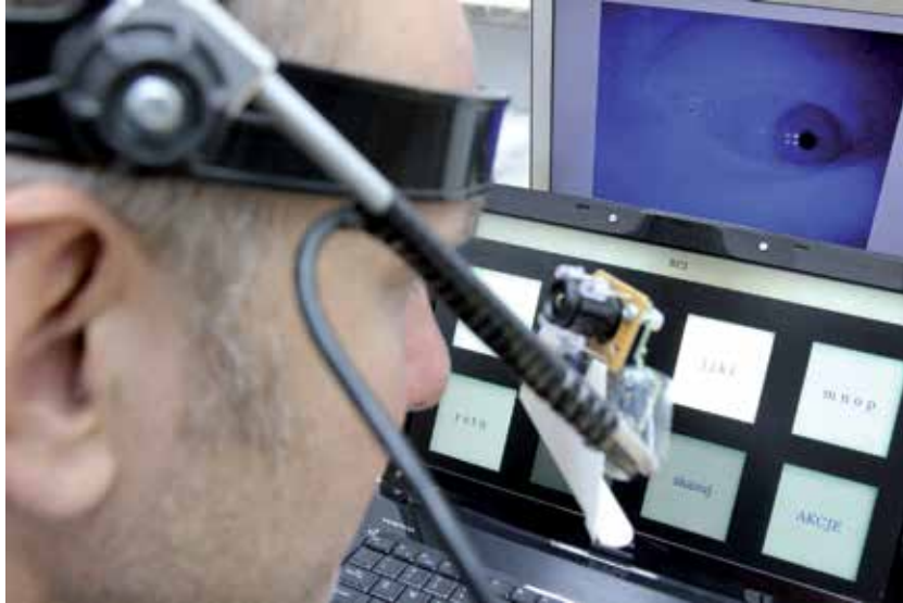
Figure 5. The first eyetracker based upon the EyeWriter project instructions, connected to the OpenBCI interface
