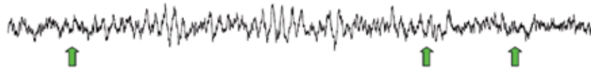
Figure 1. Sample few seconds recording of the electroencephalogram (EEG), that is potential difference between two electrodes placed on the surface of the skull. Green arrows mark the time occurrences of repetitive stimuli
