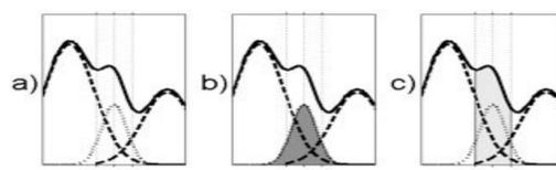
Possible improvement resulting from the MMP preprocessing stems from the uncertainty principle in signal analysis (left): (a) hypothetical spectrum resulting from presence of three different frequencies (b) actual energy estimated by MP (in case the oscillations were correctly modeled by Gabor functions) (c) energy of the structure estimated by spectral integral within predefined band.
