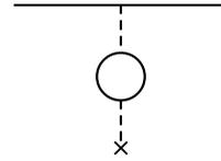
Figure 2. Diagram corresponding to the Vacuum polarization at one loop (Uehling potential). Dashed lines correspond to the Coulomb interaction, plain lines to the electron wavefunction and the cross to the interaction with the nuclear charge.
