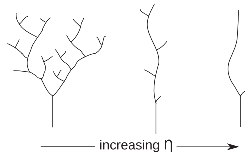
Fig. 9. Illustration of the ramified structure for increasing growth exponent \eta .
