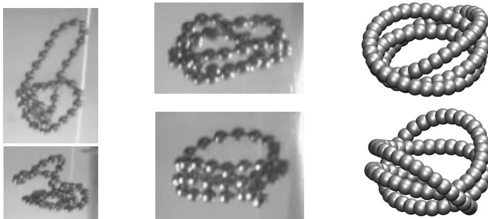
FIG. 3: Snapshots of sedimenting \mathcal{T}_{3,2} knot from experiment (initial configuration: left column, swirling: middle column) and simulation (right column, N = 90 ). Gravity points downwards.
