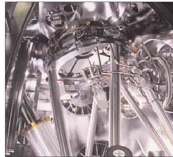
Figure 2. This engineering prototype of the engineering test stand (ETS) illuminator shows the LP light source and the C1 condenser assembly (top center). Small trapezoidally shaped doors protect the six C1-mirror petals when the ETS is not in operation. The entire condenser weldment, which also holds C2 and C3, is isolated from its environmental chamber to eliminate motion and vibration from the vacuum pumps. (Photo courtesy of Sandia National Lab)
