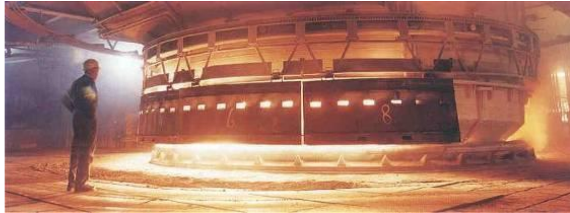
Figure 1: Schematic representation of a furnace for production of metallurgical grade silicon. Reproduced from Schei A, Tuset J, Tveit H, Production of High Silicon Alloys , Tapir forlag, Trondheim (1998).
