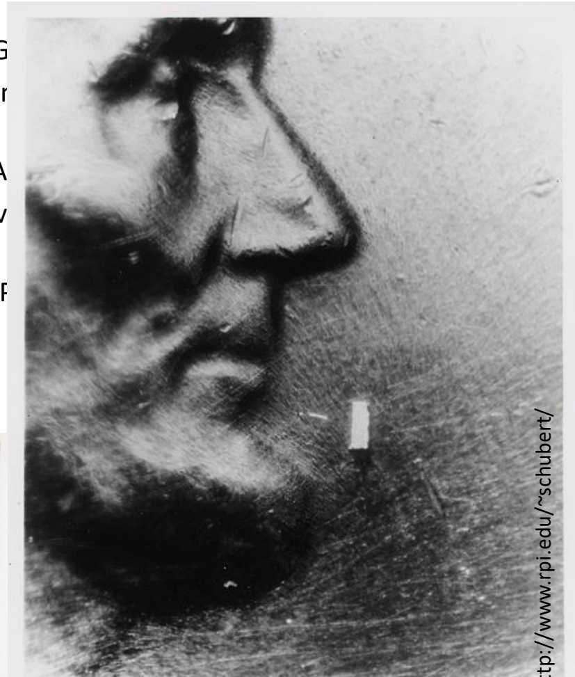
HONEST, ABE — IT'S A LASER! This new semiconductor laser, designed by Bell Laboratories scientists Izo Hayashi, Morton Panish, P. W. Foy and S. Sumski, is about 15 thousandths of an inch long by three thousandths of an inch wide. A power source no larger than a dry cell battery will operate this laser — the first of its kind to run continuously at room temperature.
