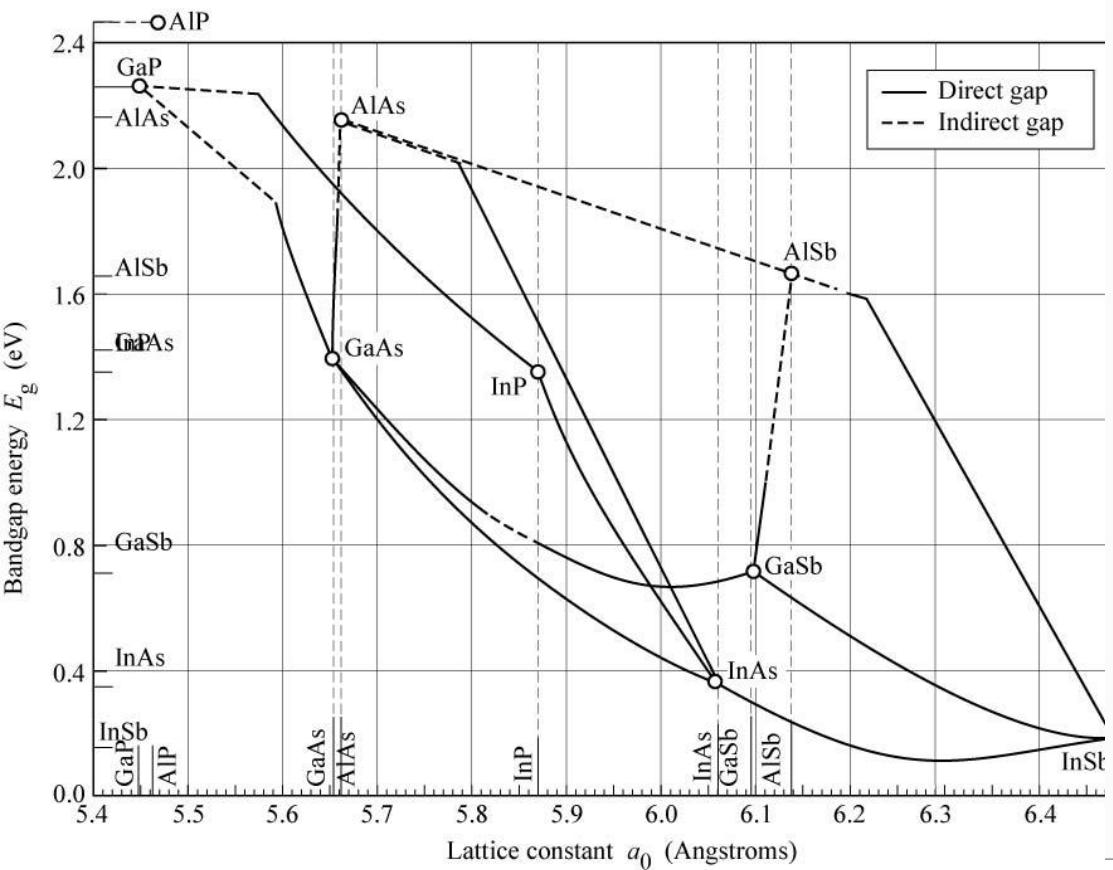
Fig. 12.6. Bandgap energy and lattice constant of various III-V semiconductors at room temperature (adopted from Tien, 1988).
