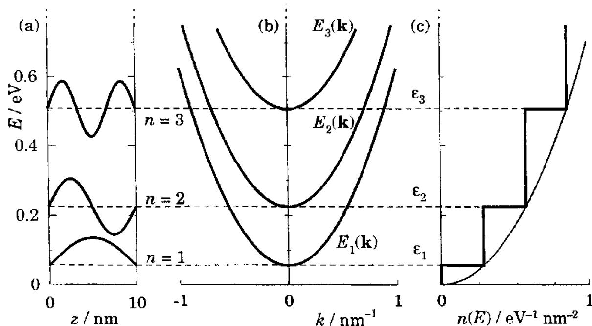
**FIGURE 4.7.** (a) Potential well with energy levels, (b) total energy including the transverse kinetic energy for each subband, and (c) steplike density of states of a quasi-two-dimensional system. The example is an infinitely deep square well in GaAs of width 10 nm. The thin curve in (c) is the parabolic density of states for unconfined three-dimensional electrons.
