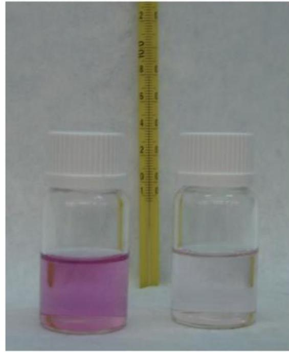
Figure 1. Bistability of a suspension of the title nanoparticles in octane: in the low-spin state (left) and in the high-spin state (right).
