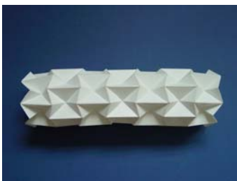
Fig. 1 A fold pattern for deployable tube.
