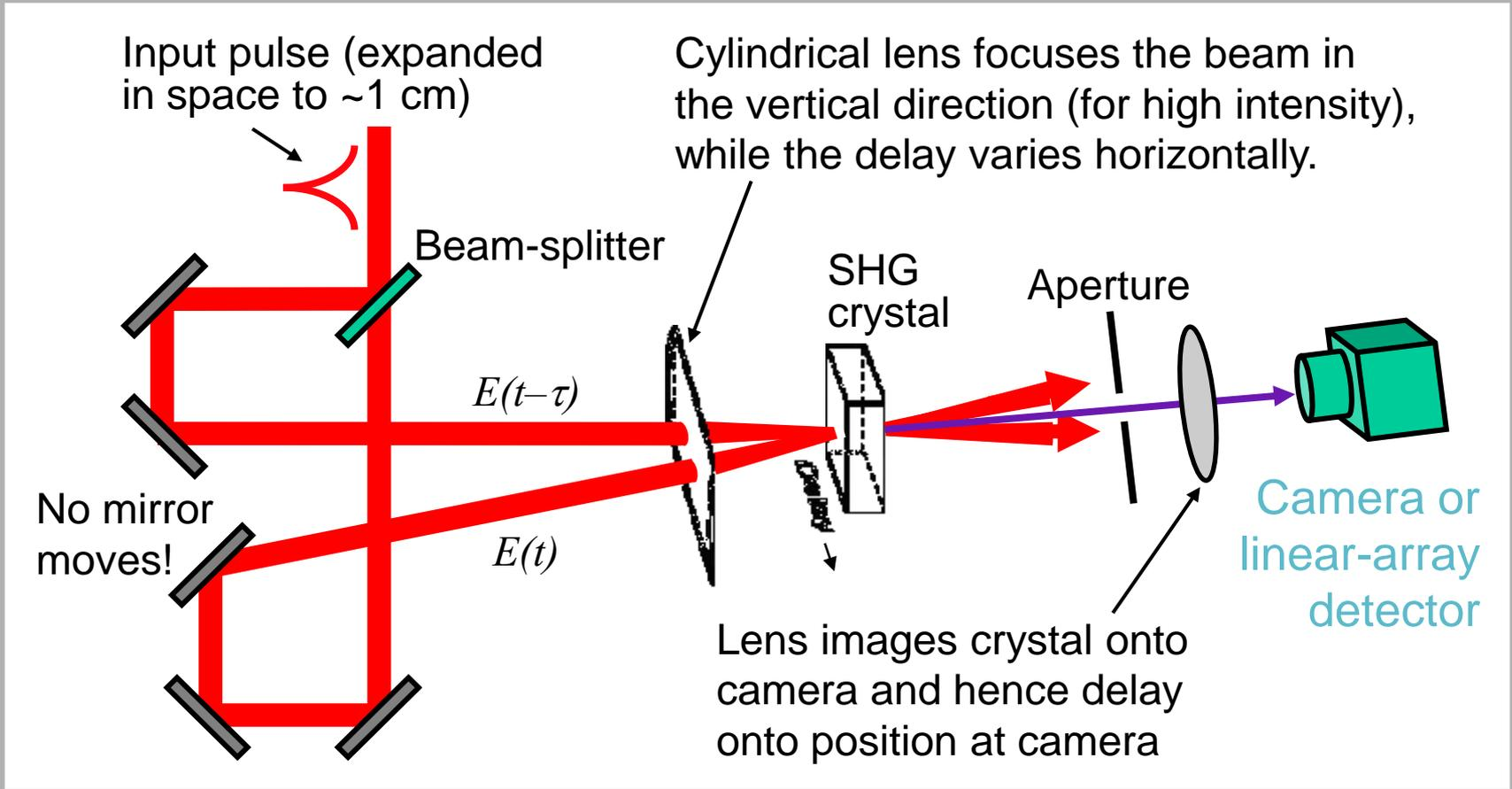
The beam must have constant intensity vs.  $x$  to avoid biases.
