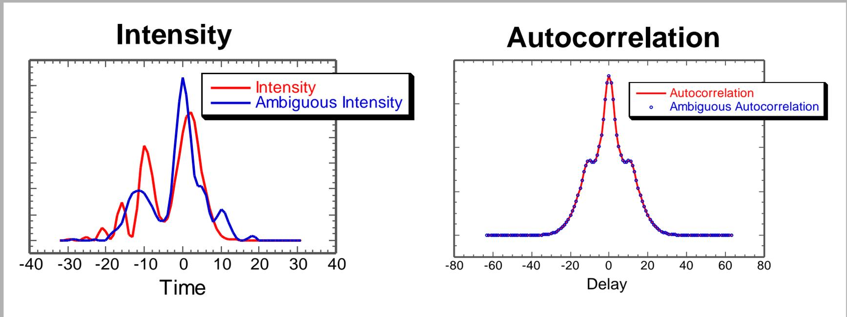
An autocorrelation typically corresponds to more than one intensity. Thus the autocorrelation does not uniquely determine the intensity.
