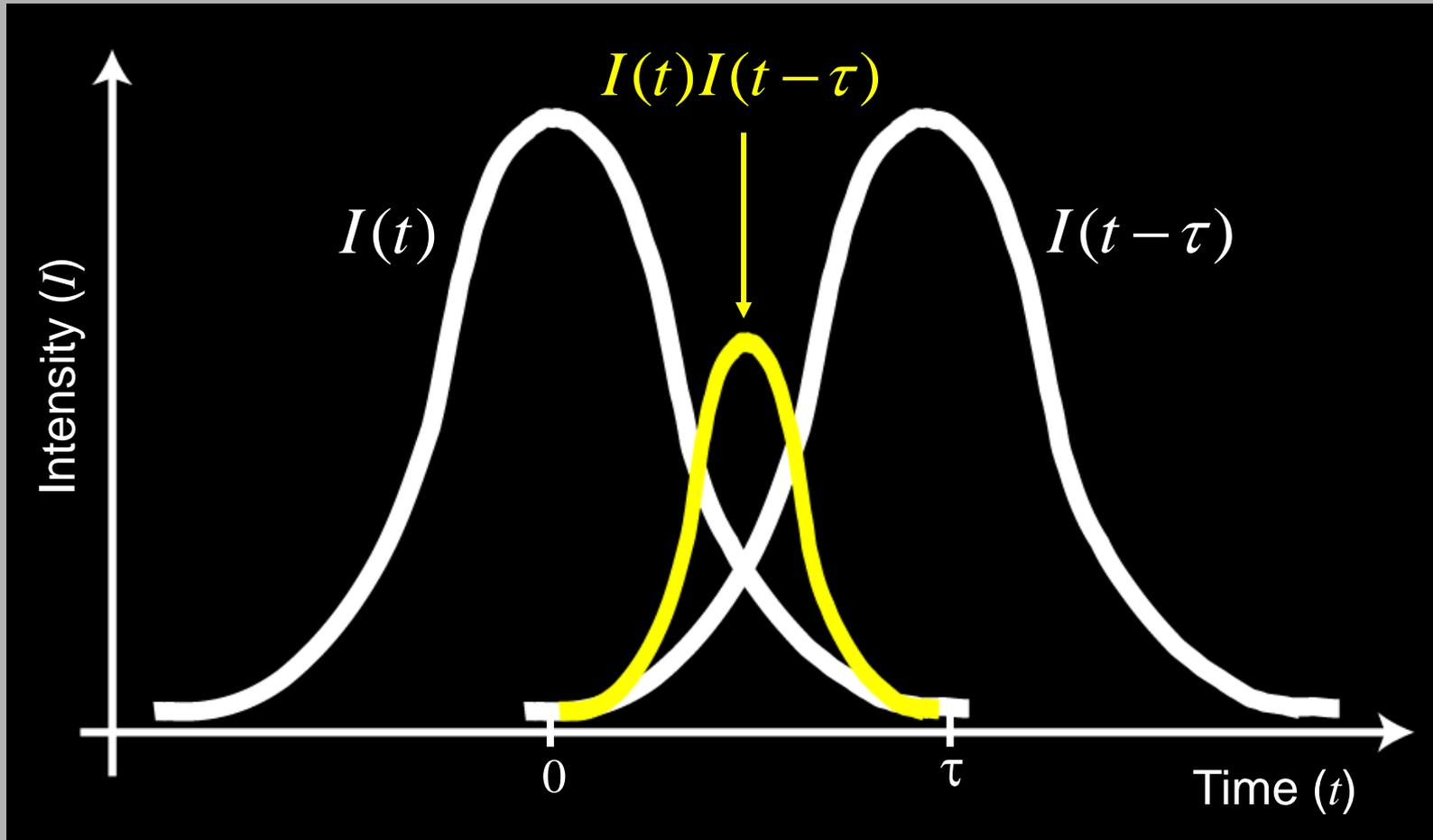
Varying the delay yields varying overlap between the two replicas of the pulse. The intensity autocorrelation is only nonzero when the pulses overlap.
