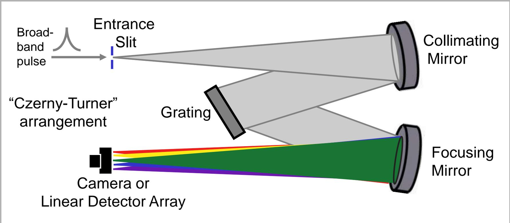
"Imaging spectrometers" allow many spectra to be measured simultaneously, one for each row of a 2D camera.
