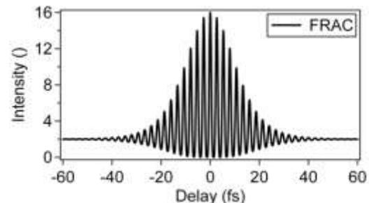
Pulse with cubic spectral phase
