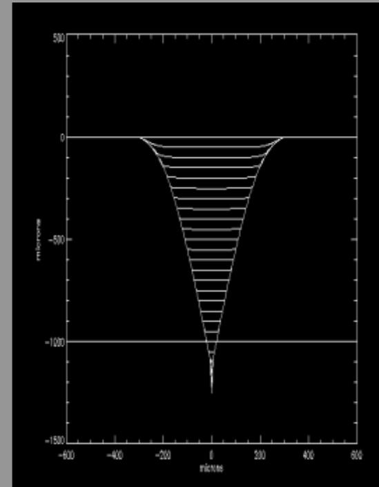
**Numerical simulation of hole drilled in human dentin by train of 350 fs pulses.**
