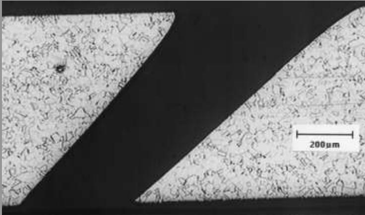
One of the main features is very localized energy deposition resulting in low collateral damage, allowing high precision material drilling.
