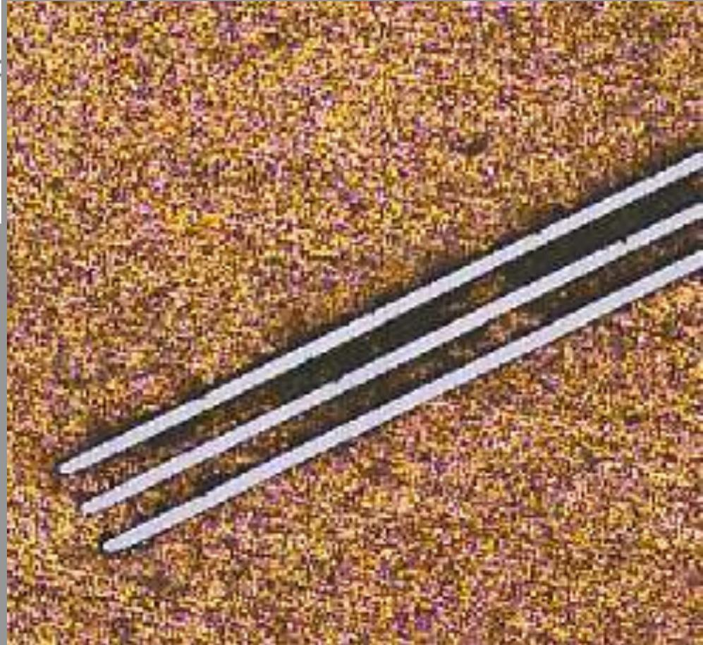
40  $\mu\text{m}$  slits in 100  $\mu\text{m}$  thick zirconia
