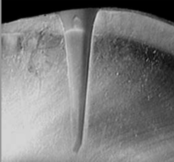
**Cross section of a conical hole drilled in tooth by a fs laser system. With no thermal shock, there is no collateral damage to adjacent tissue.**
