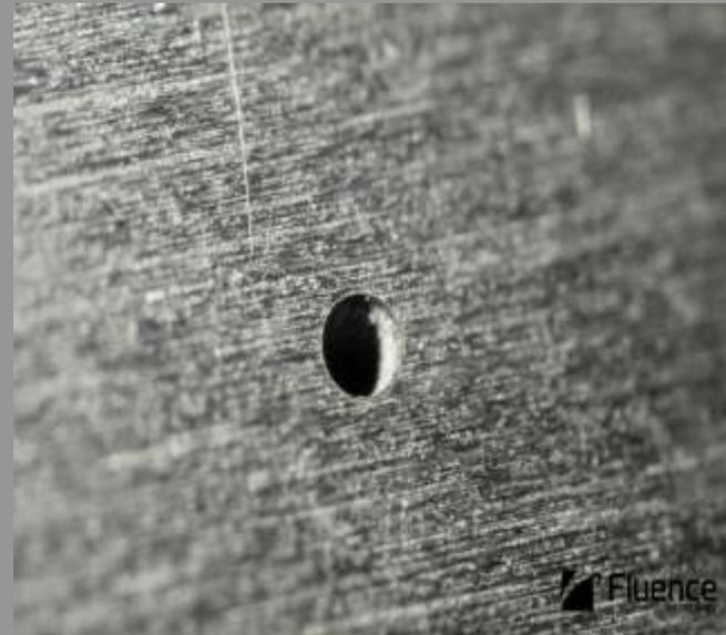
220 micron diameter hole in an aluminium alloy
