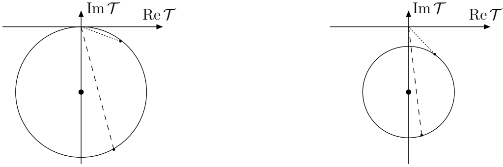
Figure 7.3: Partial amplitudes of the elastic scattering must lie on the Argand circles: if inelastic channels are closed, i.e. if R_j^2(s) = 0 , (left) the radius of the circle is s/2N_{\lambda_1\lambda_2}\sqrt{\lambda(s, m_1^2, m_2^2)} ; if inelastic channels are open (right) it is smaller. Short-dashed lines show possible partial elastic scattering amplitudes in a weakly coupled theory (small corrections in the perturbative expansion) whereas the long-dashed ones illustrate elastic scattering amplitudes typical for a strongly coupled (nonperturbative) theory.
