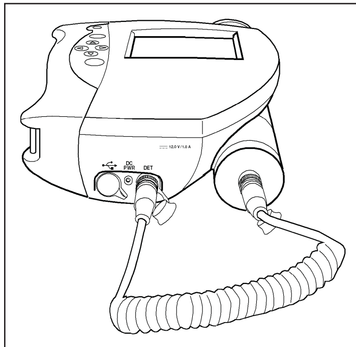
Figure 93 Connecting a Gamma Probe
