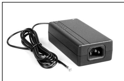
Figure 97 The ac/dc Converter
