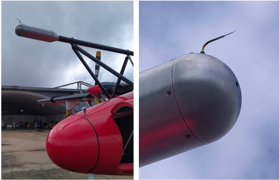
Figure 2.7: UFT-2B mounted on the BAT probe on TO. Pictures taken by M. Posyniak.
