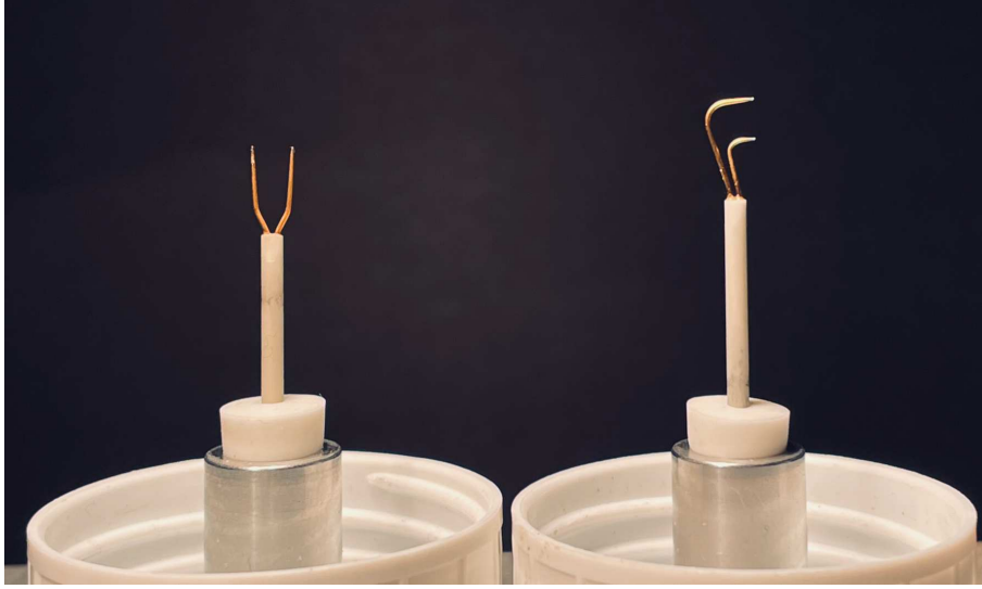
Figure 2.1: UFT-2A (left) and UFT-2B (right) head sensors. Both are topped with a tungsten wires ( 2.5\text{ }\mu\text{m} thick, 3 mm long) spanned on an miniature industry standard wire probes by DANTEC®.
