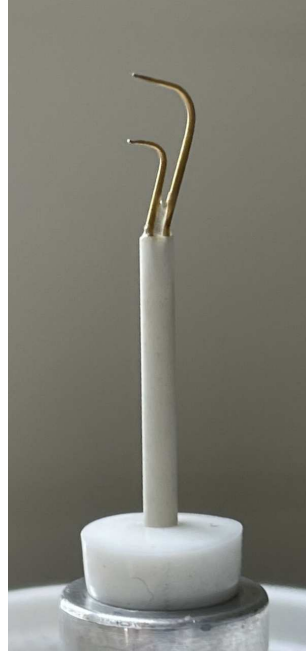
Figure C.1: UFT-2B head sensor. A parallel to the mean flow, tungsten wire ( 2.5\ \mu\text{m} thick, 3 mm long) spanned on miniature industry-standard wire probe by DANTEC ® .
