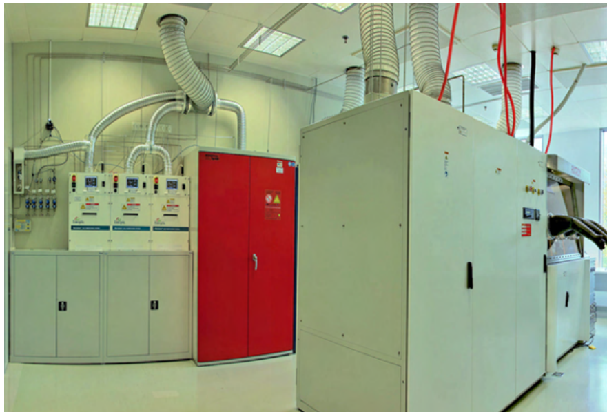
Figure 3.2: A photo of MOVPE setup at the Faculty of Physics, University of Warsaw.
