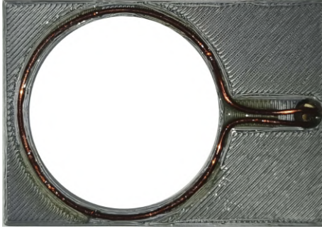
Figure 4.5: Photo of the single-loop wire in the 3D-printed housing used as an antenna for the calibration of the magnetic field.
