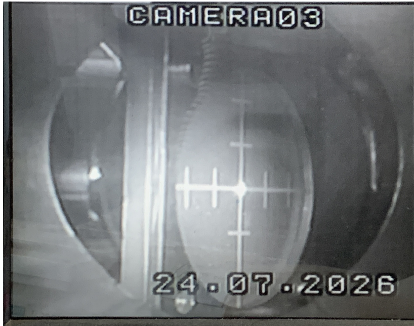
Figure 3.2: Photograph of the beam spot image on the beryllium oxide window.
