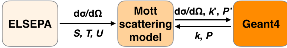
Figure 5.1: Block diagram illustrating the implementation strategy of the new interaction model in Geant4; d\sigma/d\Omega is the cross section, S, T, U are the functions determining the polarization transfer, k is the momentum, P is the polarization.
