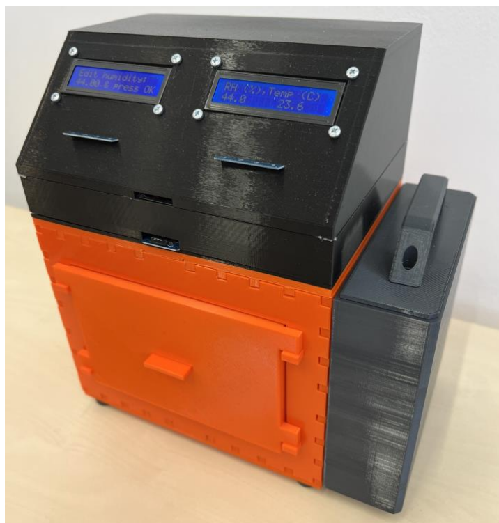
Figure 4.5 Climate chamber with controlled humidity for studies of perovskite hydration dynamics. The chamber dimensions: 20cm x 15cm x 30cm.
