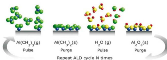
Figure 4.2 Scheme of the ALD deposition cycle 152 .
