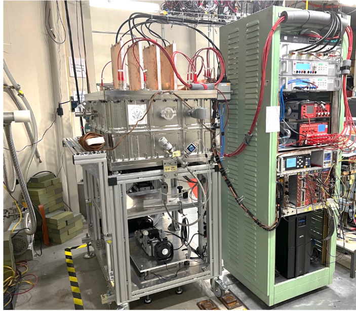
Figure 3.1: A photograph of WARSAW TPC detector and its setup during the experiment at the Upper Target Room (UTR) at HI \gamma S in April 2023. The parts depicted at the photo are the WARSAW TPC detector, detector stand, and a rack full of experimental equipment. Photo by Mikołaj Ćwiok, University of Warsaw.
