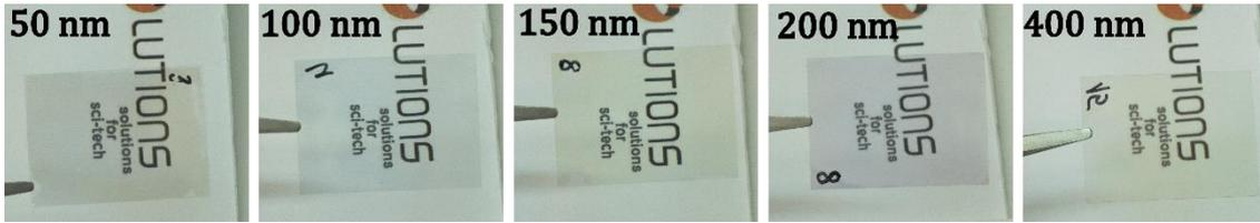
**Figure 53. Real appearances of the samples with different thicknesses.** The images were taken with the same camera setup and lighting conditions. The white piece of paper for comparison.
