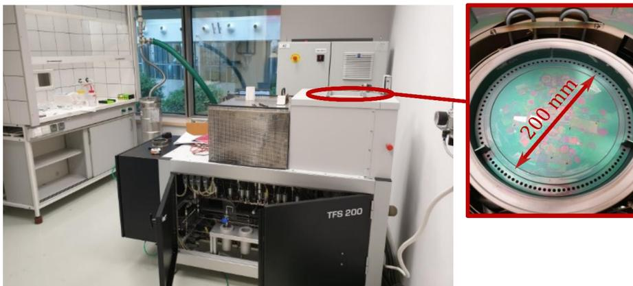
**Figure 28. ALD setup photo.** The inset shows the reaction chamber which spans over 200 mm in diameter.
