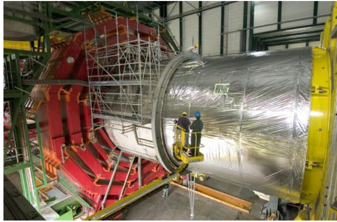
Figure 27: The picture presents the central device around which the CMS experiment is built: the superconducting magnet. [40]
