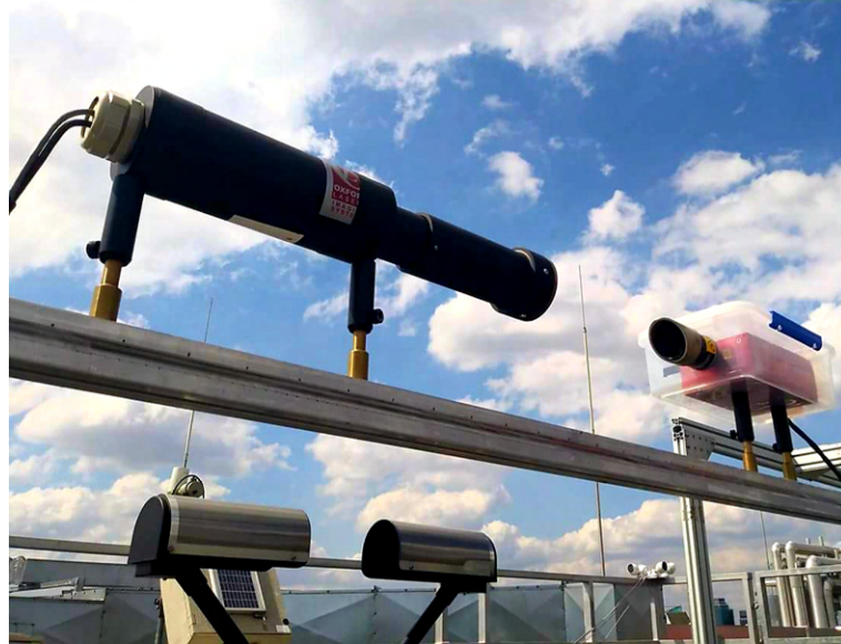
Figure 5.2: “VisiSize D30” shadowgraph instrument (front) and “OTT Parsivel 2 ” laser disdrometer (back) deployed next to each other at Meteo-station on the rooftop of the Institute of Geophysics, University of Warsaw (IGF-UW).
