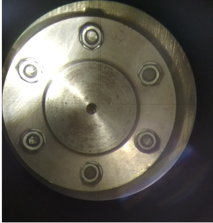
Figure 3.7: MWPC with a diaphragm mounted for the geometrical correction measurement.
