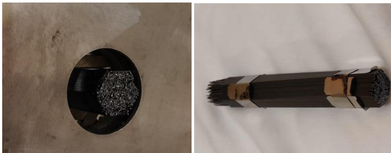
Figure 11. (left) example of stacked structure is shown on the apparatus used to stack, (right) final sealed stack of preform B.
