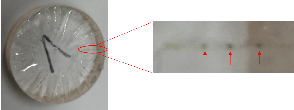
Figure 35. Micro-lenses holder used for the optical polishing with a zoom showing the lenses, of the final result after polishing (red arrows).
