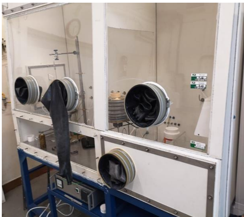
Figure 15. Glove box used for the synthesis of tellurite glasses under a protected atmosphere.
