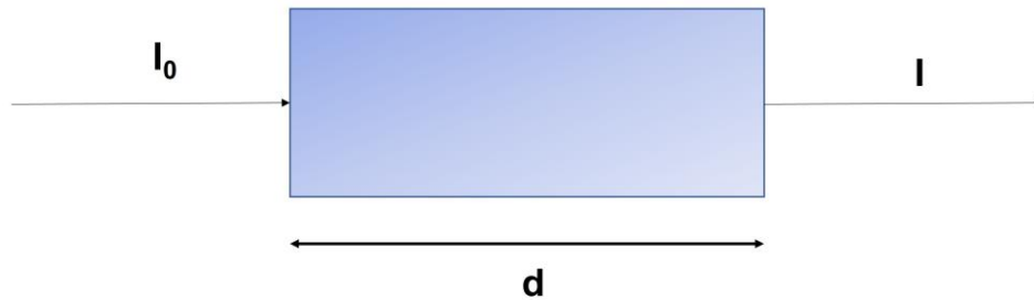
Figure 6. Attenuation of incident light propagating through a medium with a length d .
