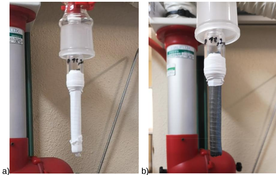
Figure 14. a) Airtight Teflon cladding of the stack connected to the drawing tower after the collapsing process at 335 degrees, b) Partially collapsed stack without the Teflon coat.
