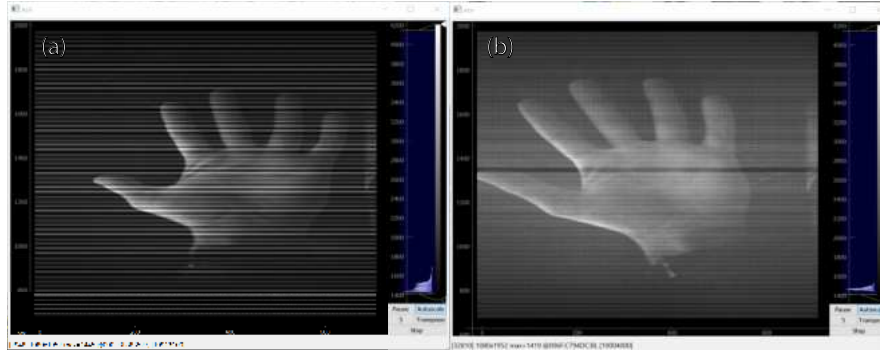
Figure 1.8: Exemplary camera frames with an objective attached instead of the image intensifier. (a) Without the ADC gain equalization (b) With the ADC gain equalized.
