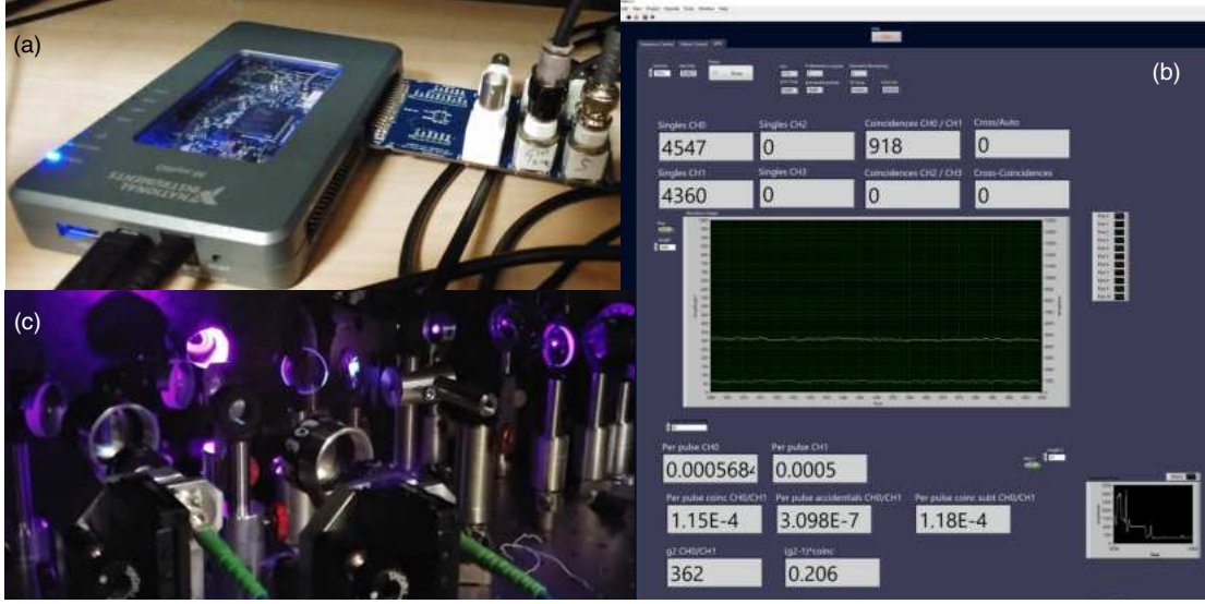
Figure 3.3: Photographs. (a) FPGA development board National Instruments myRIO-1900 with a custom input/output board attached, used for timetagging signals from single-photon avalanche photodiodes. (b) LabView program interface for live preview of the photon count statistic. (c) Fragment of the experimental setup showing a mounted BBO crystal for SPDC, blue pump filtering, and fiber coupling of the SPDC emission.
