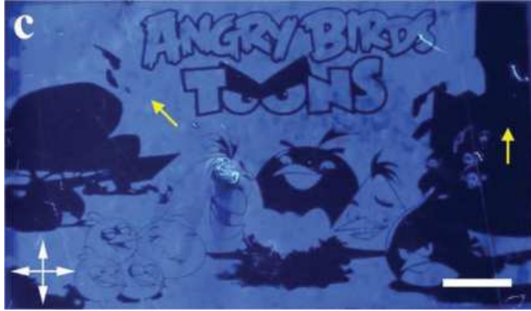
Fig. 9 POM image of a liquid crystal elastomer film fabricated using photoalignment. The alignment pattern was generated by projecting images with predefined linear polarization onto a photosensitive layer using a laser projector. White arrows indicate the polarizer and analyzer axes, and yellow arrows the local mesogen orientation. Scale bar: 3 mm. Adapted from [37].
