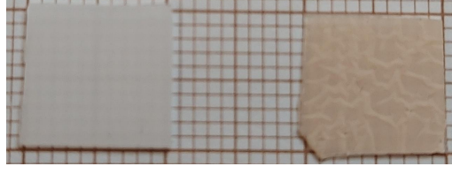
Figure 6.2: Photo of two 1 \times 1 \text{ cm}^2 rBN samples. Left: as-grown, unexposed material. Right: sample irradiated with thermal neutrons.
