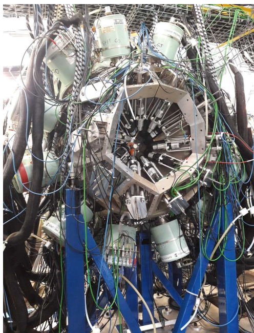
Fot. 1. Experimental setup of the \nu -ball array installed at Laboratoire de Physique des 2 Infinis Irène Joliot-Curie (ALTO, Orsay, France).
