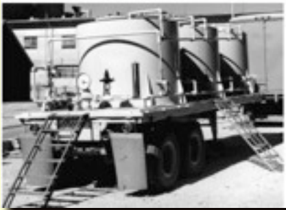
The 4500 litre tank with liquid scintillator
