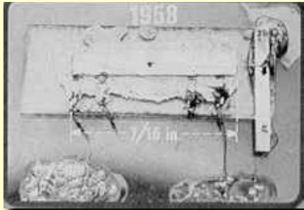
Kilby's first integrated circuit
