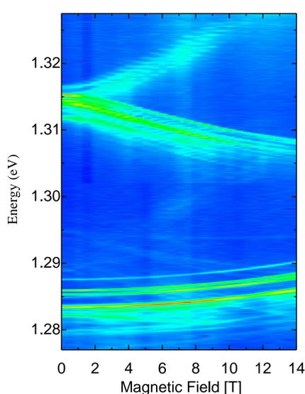
Modified single-particle Fock-Darwin spectrum well describes the emission from a single quantum dot in magnetic field
