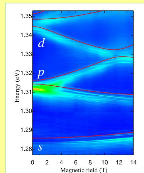
Energies of the S<sub>2</sub>, P<sub>1</sub>, P<sub>4</sub>, D<sub>1</sub> and D<sub>2</sub> emission lines plotted against magnetic field. Symbols give the experimental data. Calculated single-particle FD spectrum is shown with dotted lines. Solid lines - the excitonic FD spectrum (modified by electron-electron interaction and zero-field splitting)
