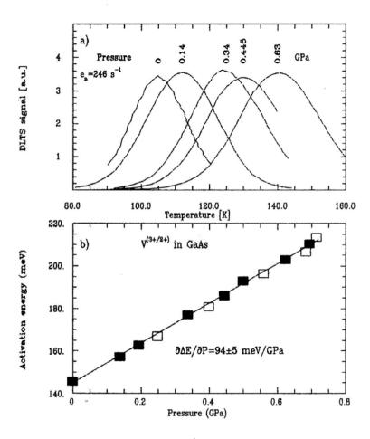
Fig. 1. a) DLTS spectra for  $V^{3+/2+}$  acceptor level in GaAs ( $\Delta E = 0.146$  eV) under hydrostatic pressure; the emission rate window  $e_n = 246 \, \mathrm{s}^{-1}$ ; b) the pressure dependence of  $V^{3+/2+}$  level activation energy; full and empty squares correspond to the values obtained with  $e_n = 246 \, \mathrm{s}^{-1}$  and  $e_n = 2470 \, \mathrm{s}^{-1}$ , respectively.
