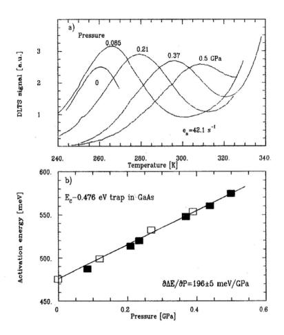
Fig. 2. a) DLTS spectra for 0.476 eV trap related to Ni<sup>2+/1+</sup> double acceptor level in GaAs under hydrostatic pressure; the emission rate window  $e_n = 42.1 \text{ s}^{-1}$ ; b) the pressure dependence of emission rate activation energy for 0.48 eV trap; full and empty squares correspond to the values obtained with  $e_n = 42.1 \text{ s}^{-1}$  and  $e_n = 246 \text{ s}^{-1}$ , respectively.
