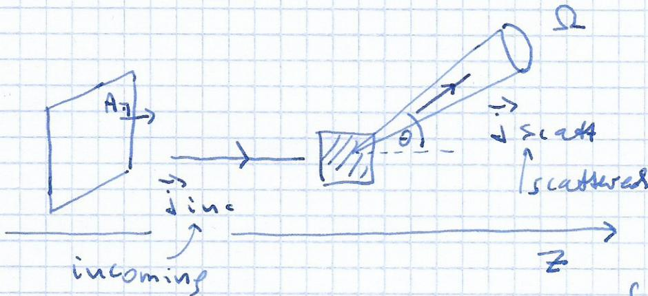
detector records number of particles scattered into a solid angle  $\Omega$
