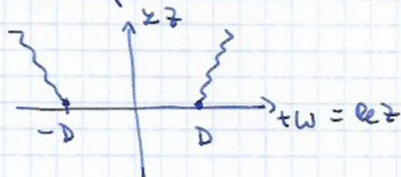
The pole moves away from the real axis down into the lower half-plane
