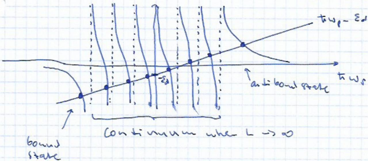
Poles  $tW_p^0 = \epsilon_k$  at  $V_k = 0$  are shifted due to finite hybridization
