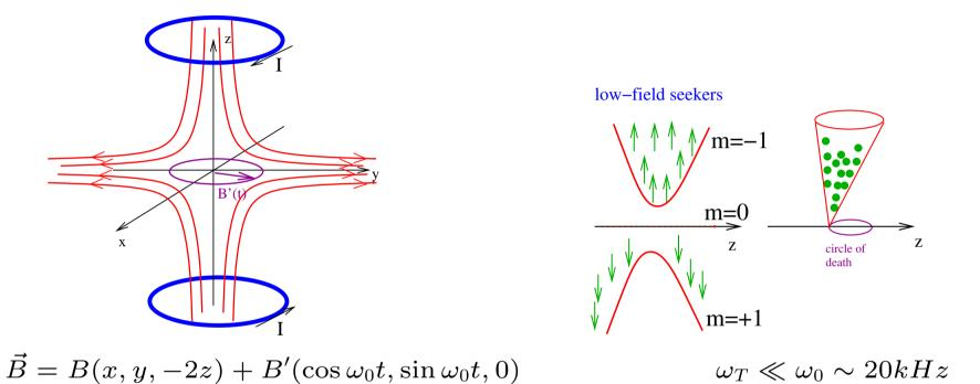
$$\bar{B}(r) = \frac{\omega_0}{2\pi} \int_0^{2\pi/\omega_0} dt B(t) \approx B' + \frac{B^2}{4B'} (x^2 + y^2 + 8z^2) + \dots$$
