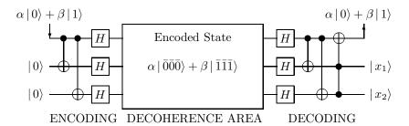
Careful inspection of the network shows that any single phase-flip  $|\bar{0}\rangle \leftrightarrow |\bar{1}\rangle$  will be corrected and the environment will be effectively disentangled from the qubits. In our particular case we obtain
