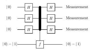
The control register, now composed out of n qubits (n=3 in the diagram above), is initially in state  $|00\cdots 0\rangle$  and an auxiliary qubit in the second register starts and remains in the state  $|0\rangle - |1\rangle$ .
