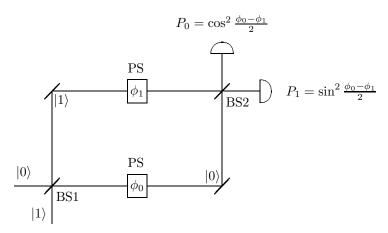
If the lower path is labeled as state  $|0\rangle$  and the upper one as state  $|1\rangle$  then the particle, initially in path  $|0\rangle$ , undergoes the following sequence of transformations
