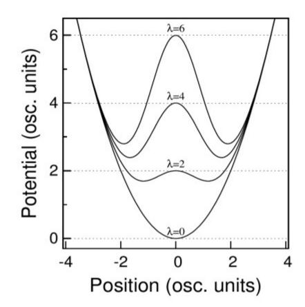
$\lambda$  – dimensionless parameter controlling the height of the potential barrier
