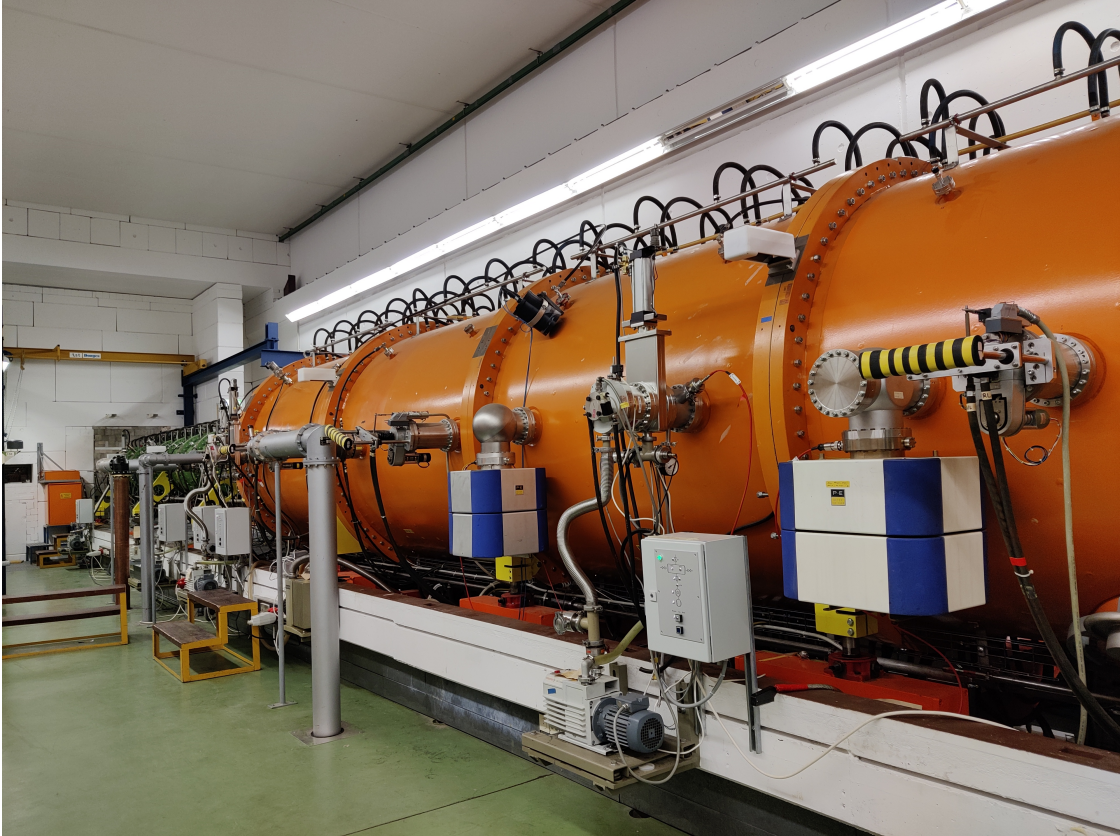
Figure 34: High Current Injection (HSI) part of UNILAC
