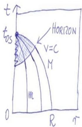
$$t_{OS} = \frac{1}{2} \left( \frac{R_G}{c} \right) \left( \frac{R}{R_G} \right)^{3/2}$$
