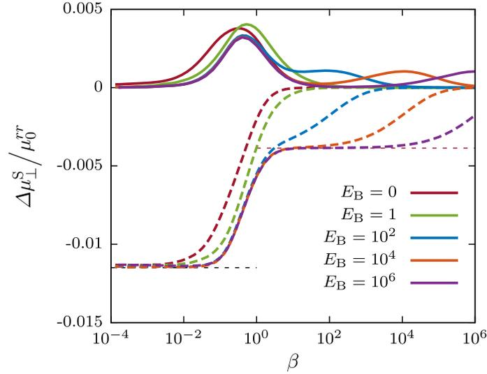
**Fig. 4** (Color online) Scaled particle self mobility corrections versus  $\beta$  for various values of the reduced bending modulus  $E_B$  for the rotational motion around an axis perpendicular to the cylinder axis. Here we take  $R = 4a$  and  $C = 1$
