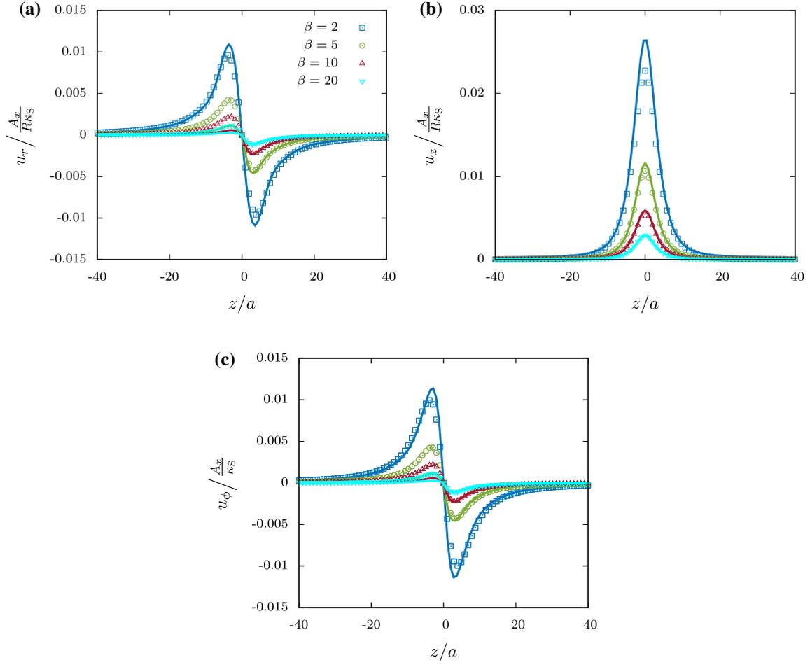
**Fig. 7** (Color online) Scaled radial (a), axial (b), and azimuthal (c) membrane displacement field versus scaled distance along the axis  $z/a$  for four forcing frequencies calculated at quarter period for  $\omega_0 t = \pi/2$  when the particle reaches its maximal radial position. Here deformations are shown in the plane of maximum deformation. *Solid lines* are the theoretical predictions, and symbols refer to the boundary integral simulation results
