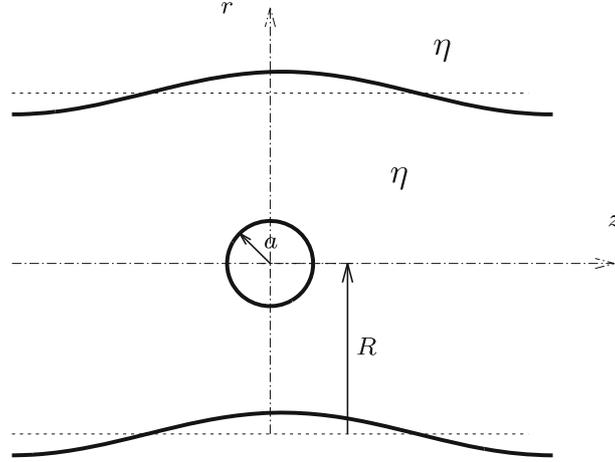
**Fig. 1** Illustration of the system setup. A small spherical particle of radius  $a$  placed at the origin rotating nearby an elastic tube of undisturbed radius  $R$
