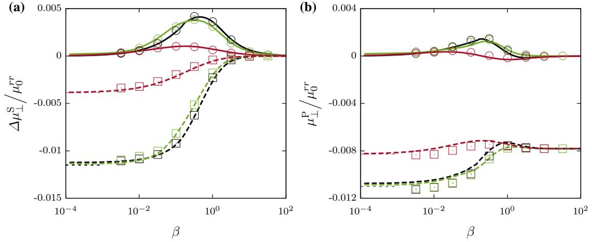
**Fig. 3** (Color online) Scaled frequency-dependent self (a) and pair (b) mobilities versus the scaled frequency  $\beta$  for the rotational motion around an axis perpendicular to the cylinder axis. The *color code* is the same as in Fig. 2
