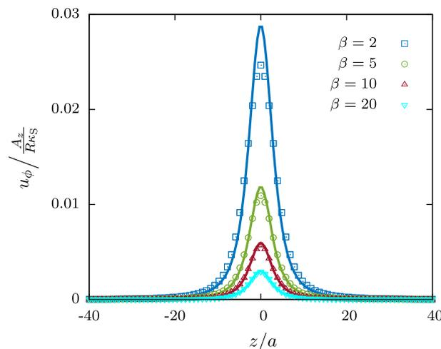
**Fig. 6** (Color online) Scaled azimuthal membrane displacements versus  $z/a$  at four forcing frequencies computed at quarter oscillation period for  $t\omega_0 = \pi/2$ . *Solid lines* are the analytical predictions, and symbols refer to boundary integral simulations
